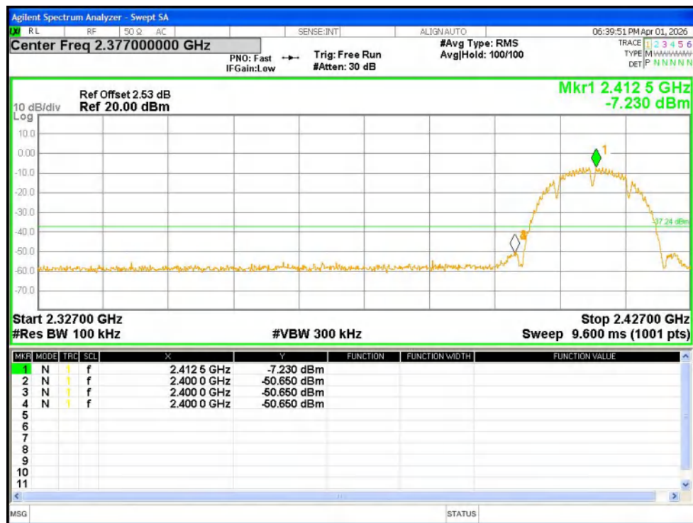
Band Edge NVNT b 2412MHz Ant1 Emission
