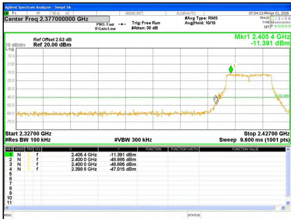
Band Edge NVNT g 2412MHz Ant1 Emission
