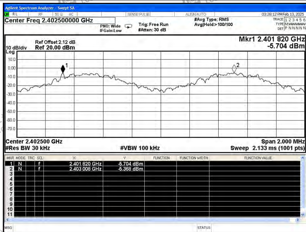
CFS NVNT 2-DH5 2402MHz Ant1
