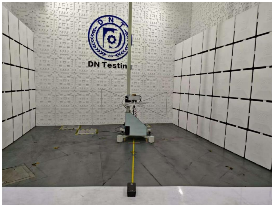
Radiated Emission Test View|(Below 1G)
