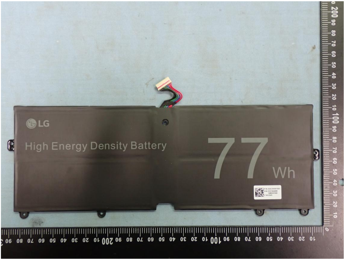
Figure 40 Battery, Front View
