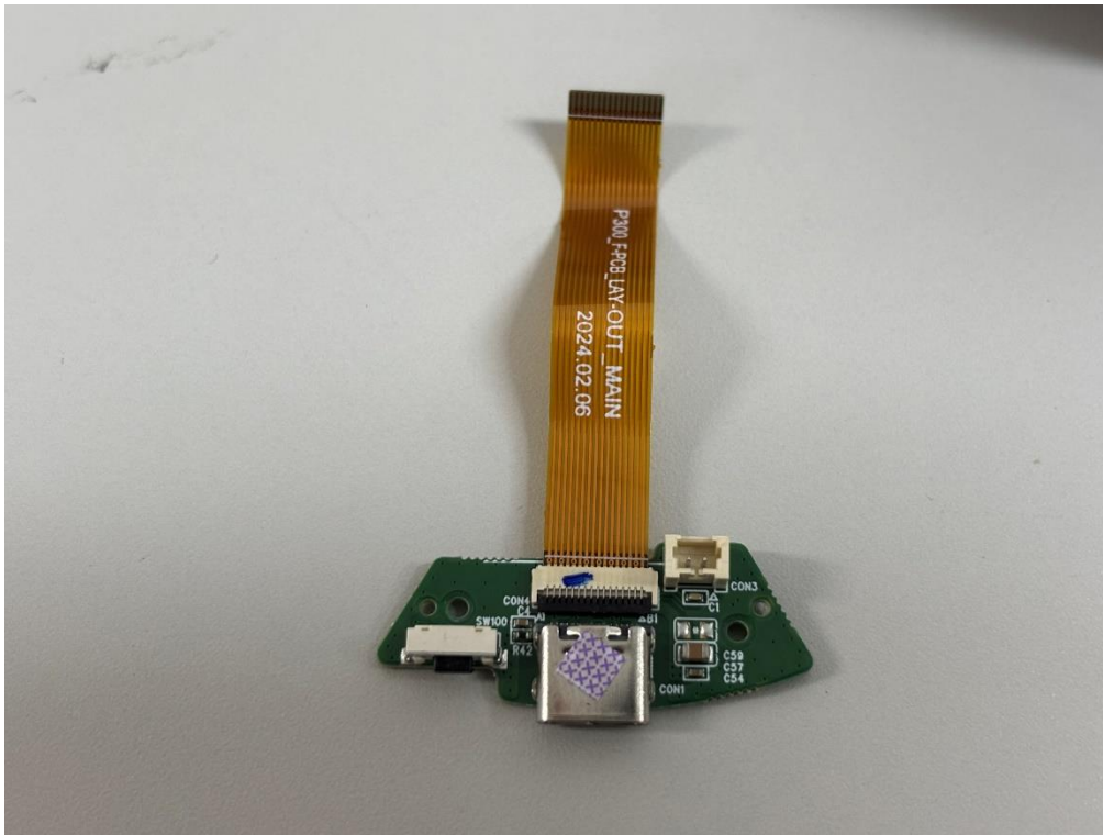
C type power Board – Front
