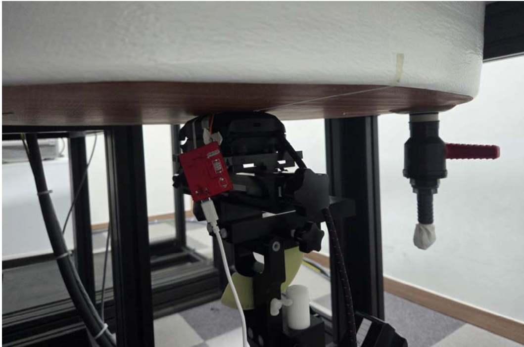
SAR Test Picture(Right), Test separation distance : 0 mm
