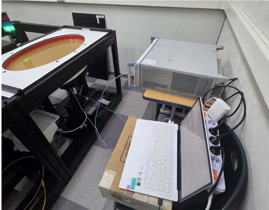
SAR Test Picture(Front), Test separation distance : 0 mm
