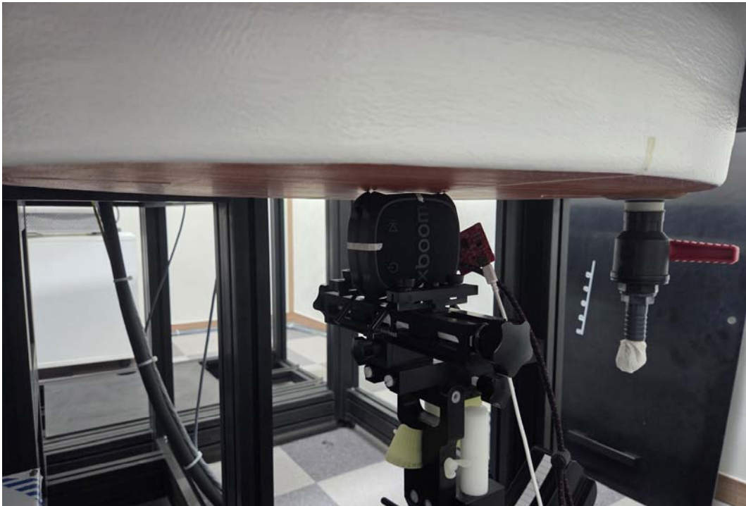
SAR Test Picture(Right), Test separation distance : 0 mm
