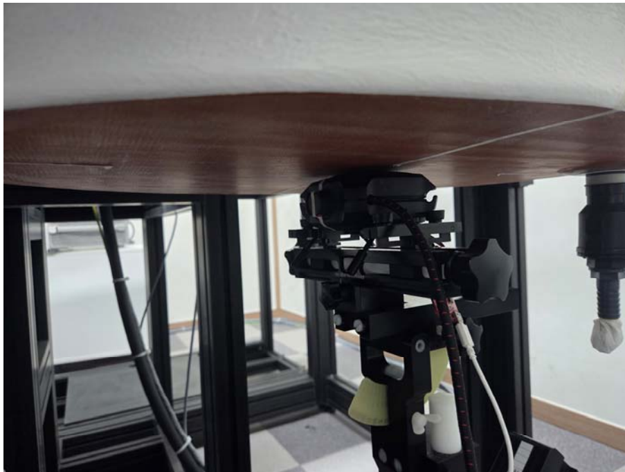
SAR Test Picture(Front), Test separation distance : 0 mm
