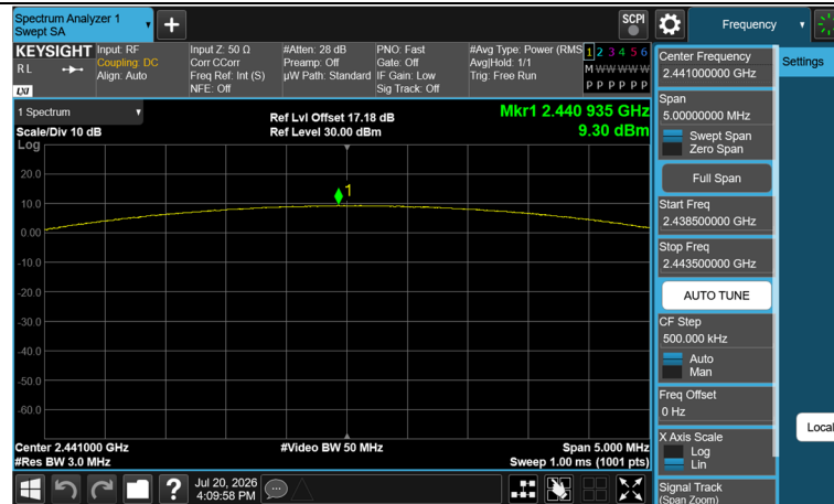
\pi /4DQPSK : Peak Power (Ch. 0)
