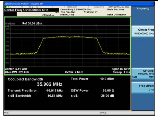
Bandwidth 40M, 802.11ac(VHT40) Ch.102
