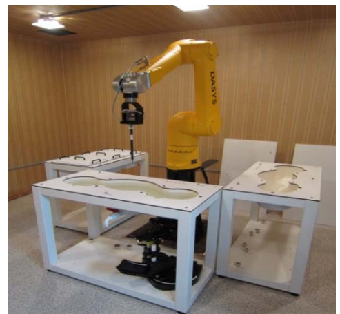
Figure E.8.1 DASY5 Test System
