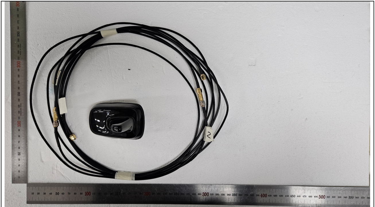
< Main Antennas + Cable >
