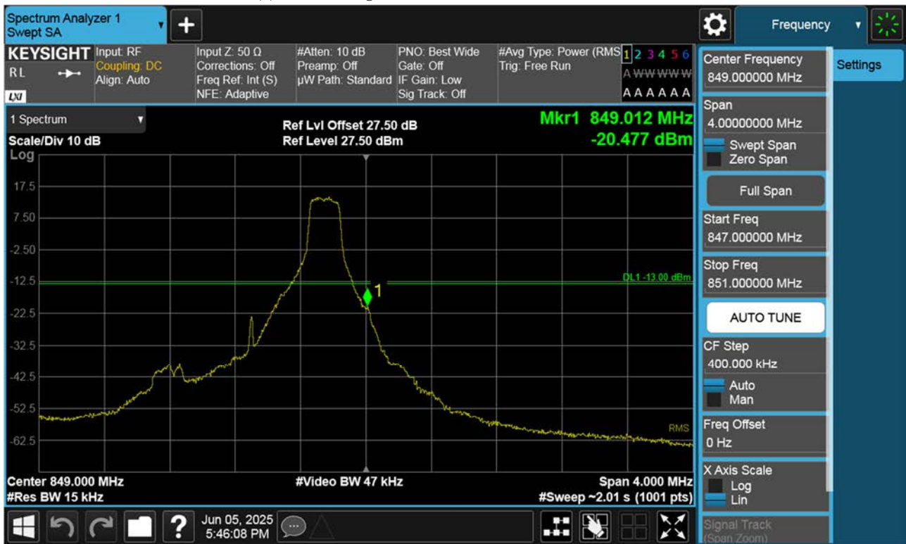
LTE B26_ Upper Band Edge Plot (1.4 M BW Ch.27033 QPSK_RB1_Offset 5)
