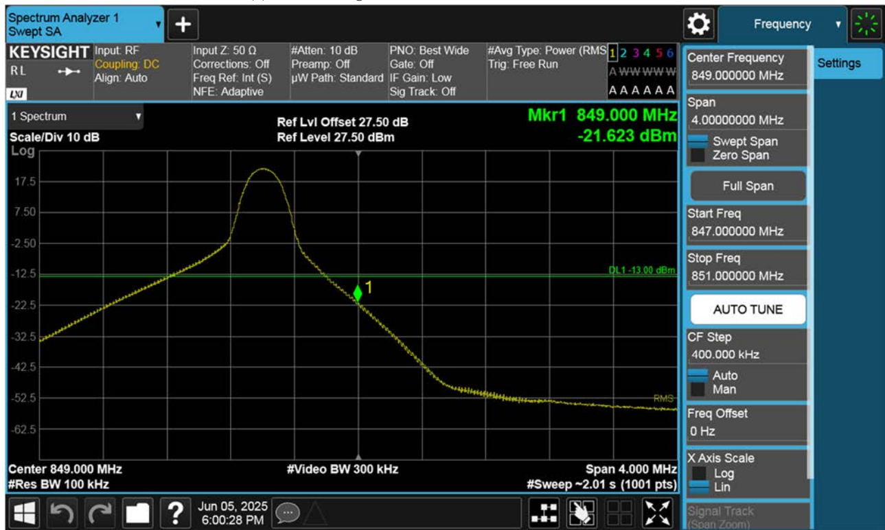
LTE B26_ Upper Band Edge Plot (10 M BW Ch.26990 QPSK_RB1_Offset 49)
