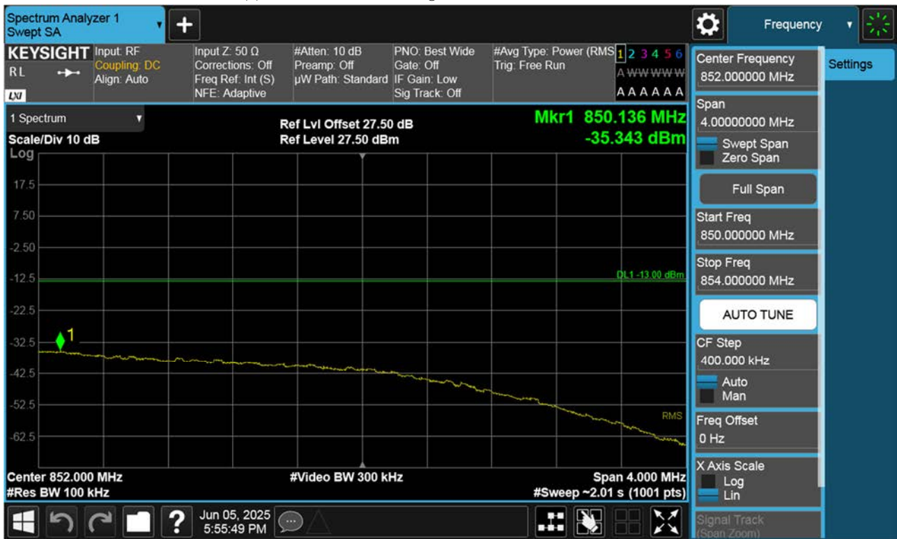
LTE B26_ Upper Extended Band Edge Plot (5 M BW Ch.27015 QPSK_RB25_0)
