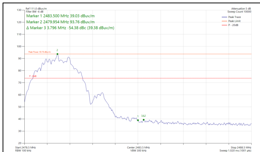
Figure 56 - CH39_UBE_LE2M, 2480 MHz, Band Edge Frequency 2483.5 MHz
