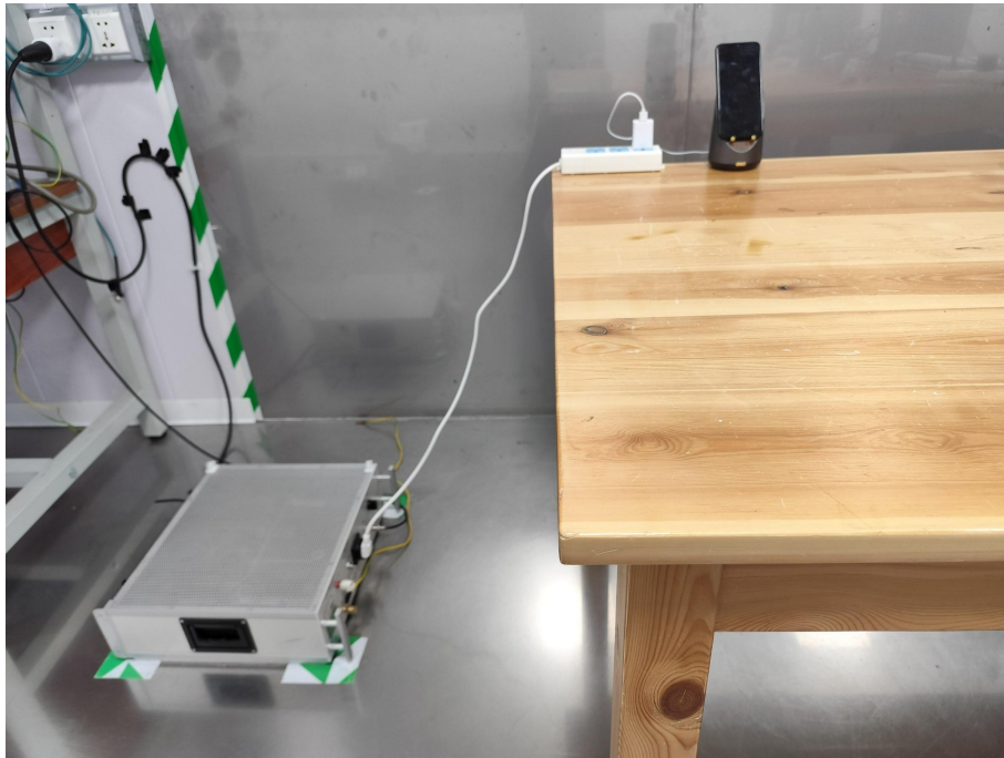
Conducted Emission at AC power line
