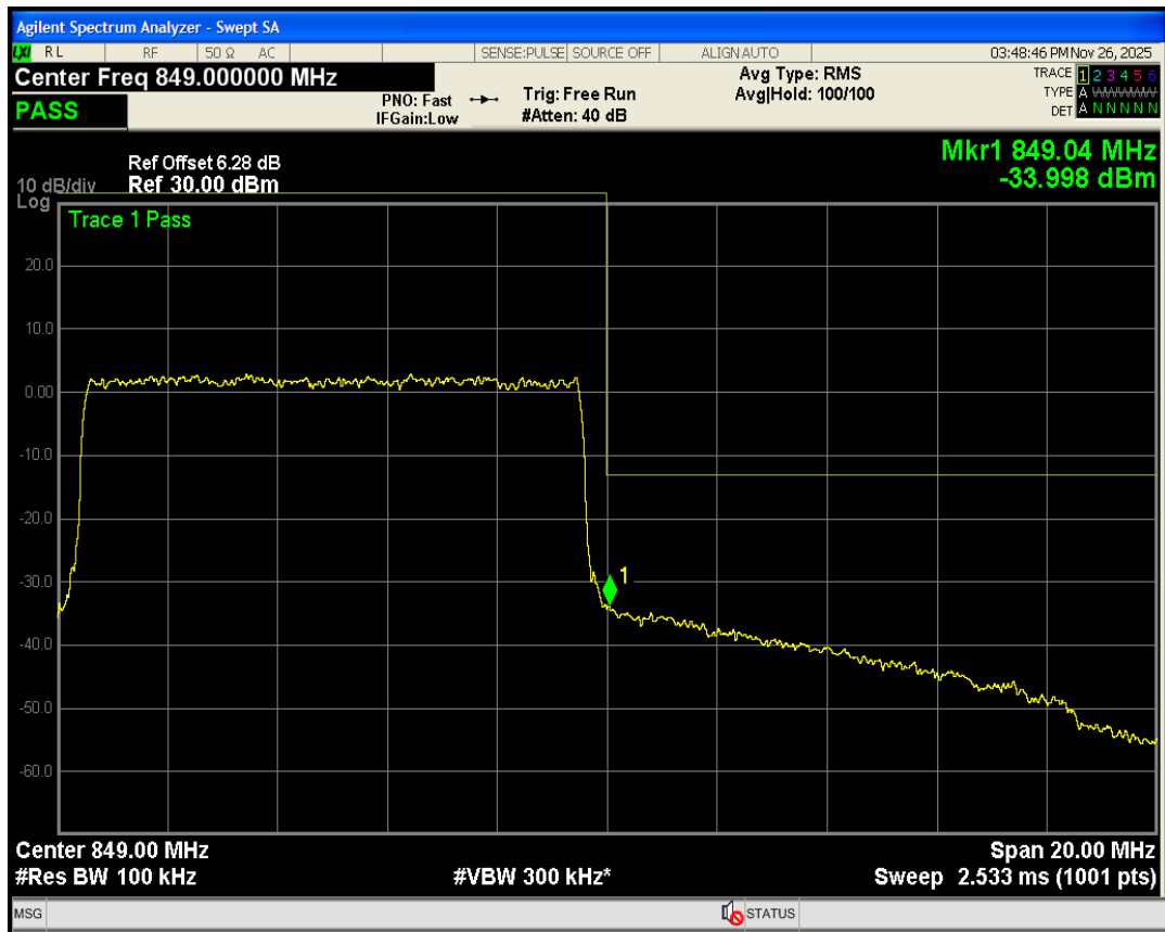
Band5 QAM16 BW=10MHz Channel=20600 RB Size=27 Position=#0
