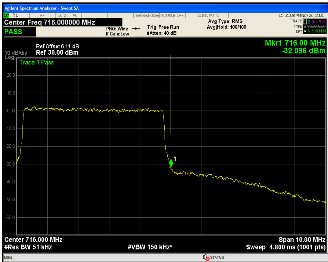
Band17 QPSK BW=10MHz Channel=23780 RB Size=50 Position=#0
