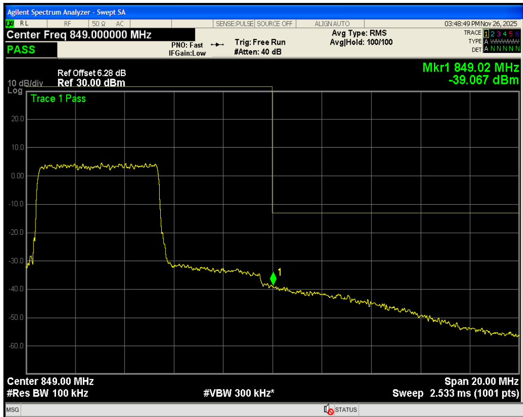
Band66 QPSK BW=1.4MHz Channel=131979 RB Size=6 Position=#0
