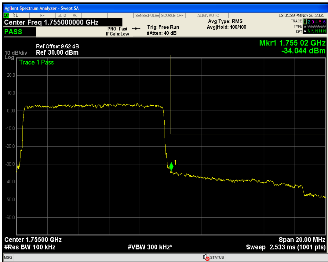
Band4 QAM16 BW=10MHz Channel=20000 RB Size=27 Position=#0
