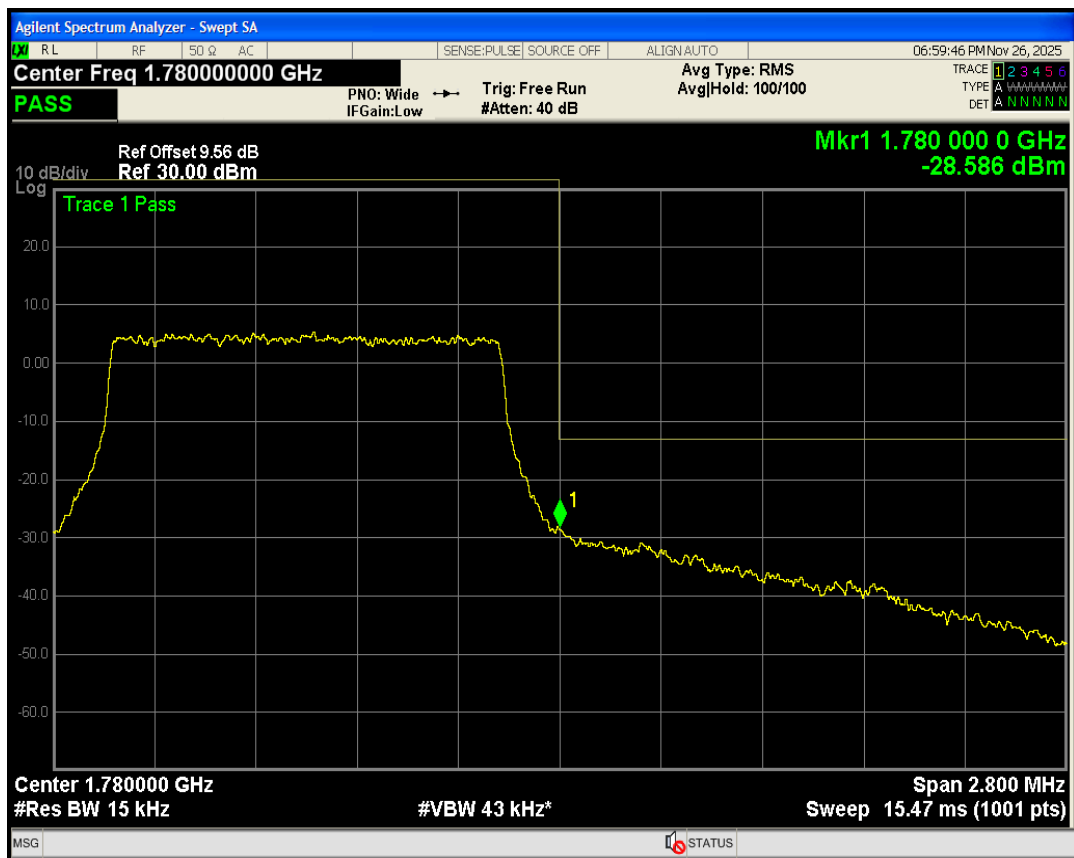
Band66 QPSK BW=3MHz Channel=131987 RB Size=15 Position=#0
