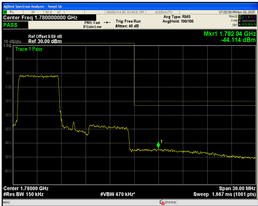
Band66 QPSK BW=20MHz Channel=132072 RB Size=100 Position=#0
