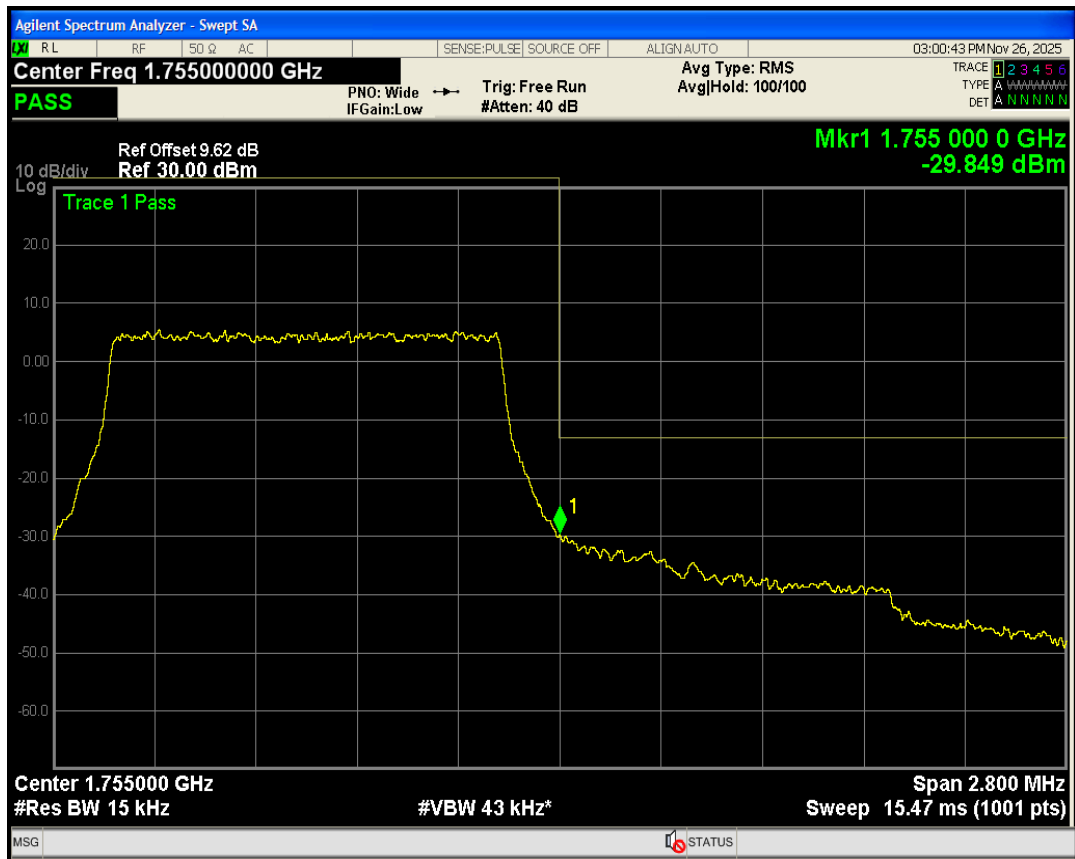
Band4 QAM16 BW=1.4MHz Channel=20393 RB Size=6 Position=#0
