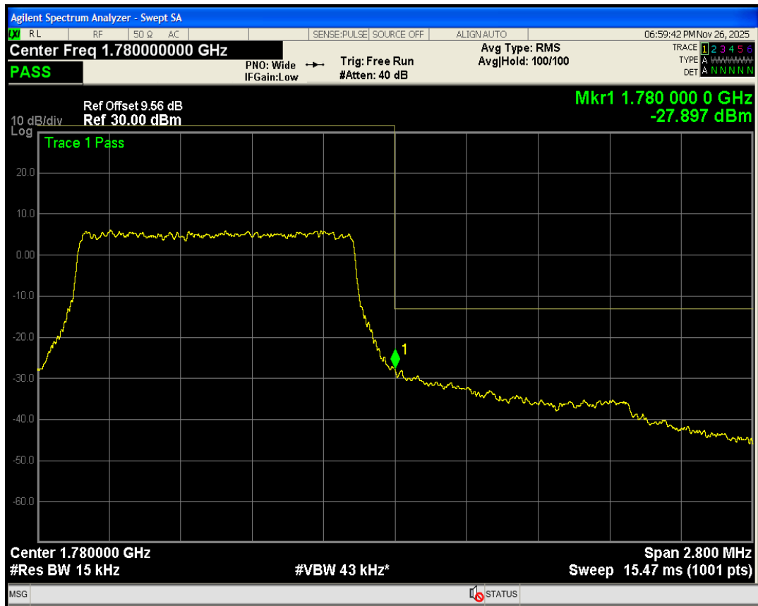
Band66 QAM16 BW=1.4MHz Channel=132665 RB Size=6 Position=#0
