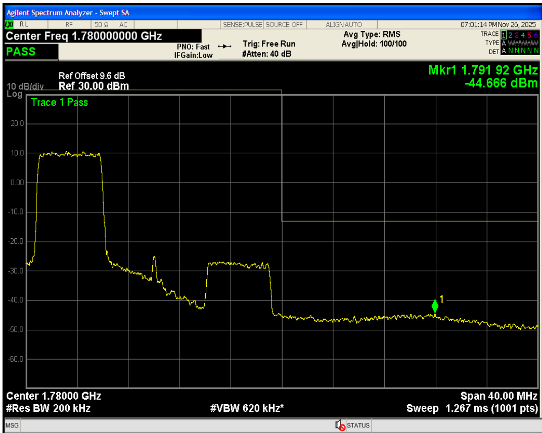
Band7 QAM16 BW=5MHz Channel=20775 RB Size=25 Position=#0
