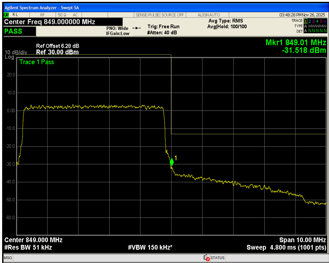
Band5 QAM16 BW=5MHz Channel=20625 RB Size=25 Position=#0
