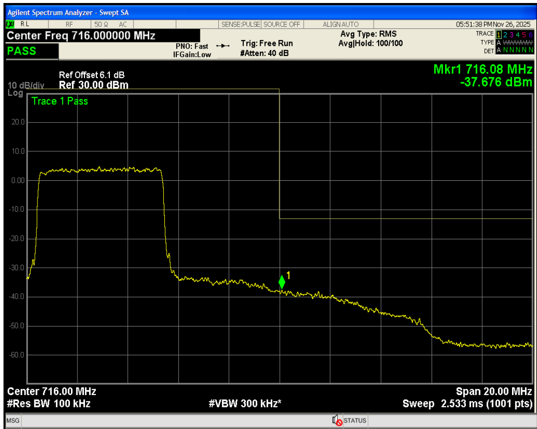
Band17 QPSK BW=10MHz Channel=23800 RB Size=50 Position=#0
