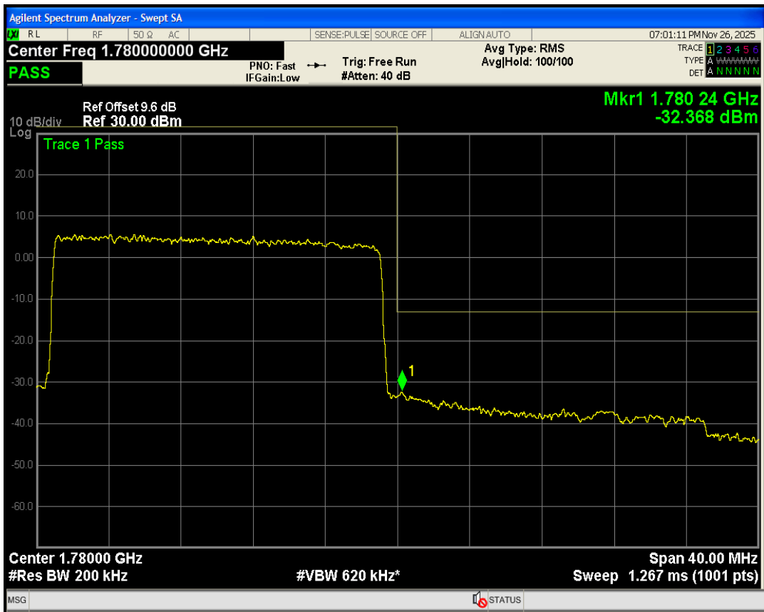
Band66 QAM16 BW=20MHz Channel=132572 RB Size=27 Position=#0
