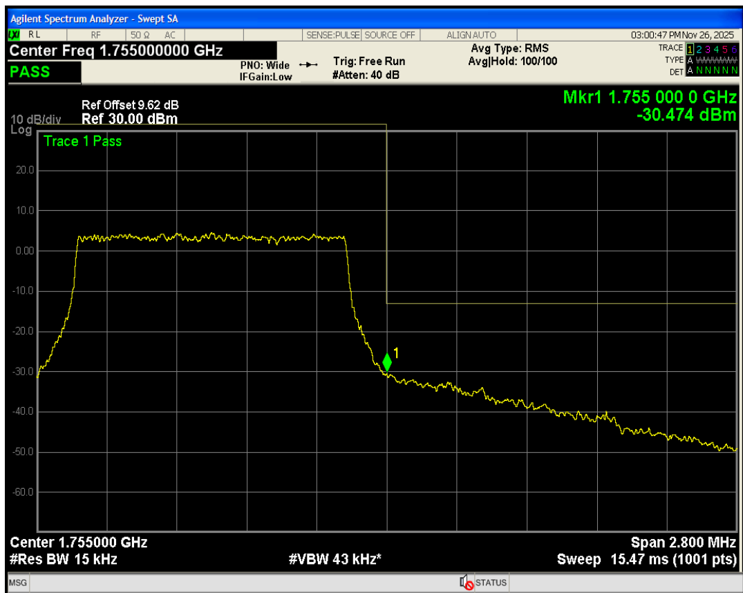
Band4 QPSK BW=3MHz Channel=19965 RB Size=15 Position=#0
