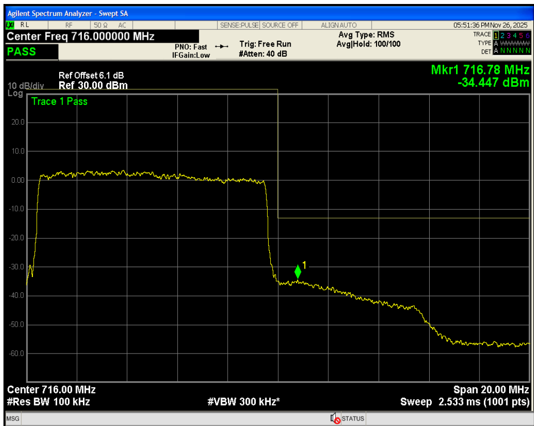
Band38 QPSK BW=5MHz Channel=37775 RB Size=25 Position=#0
