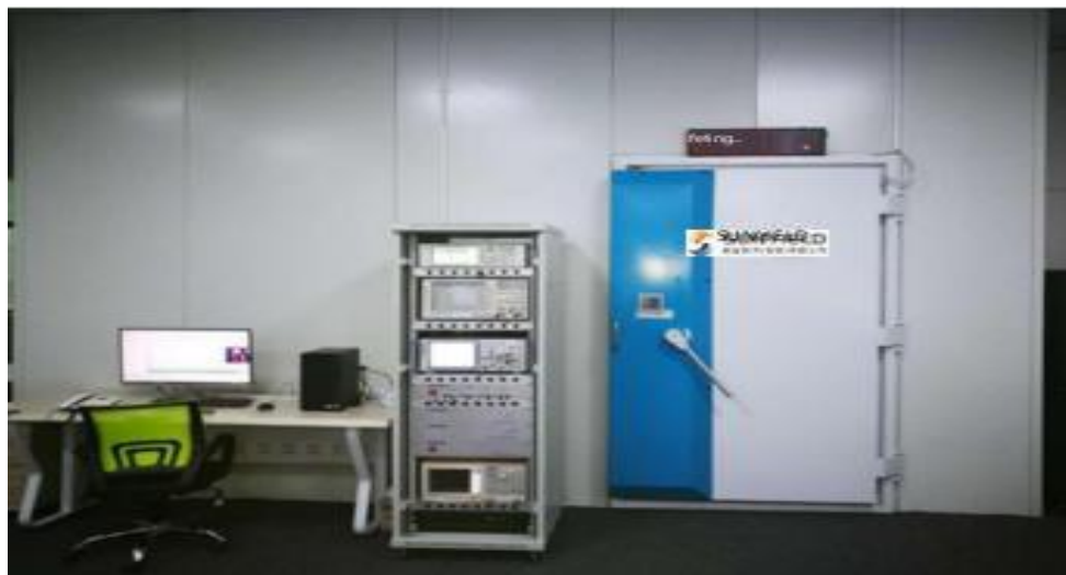
External diagram of microwave darkroom (darkroom+cabinet equipment)
