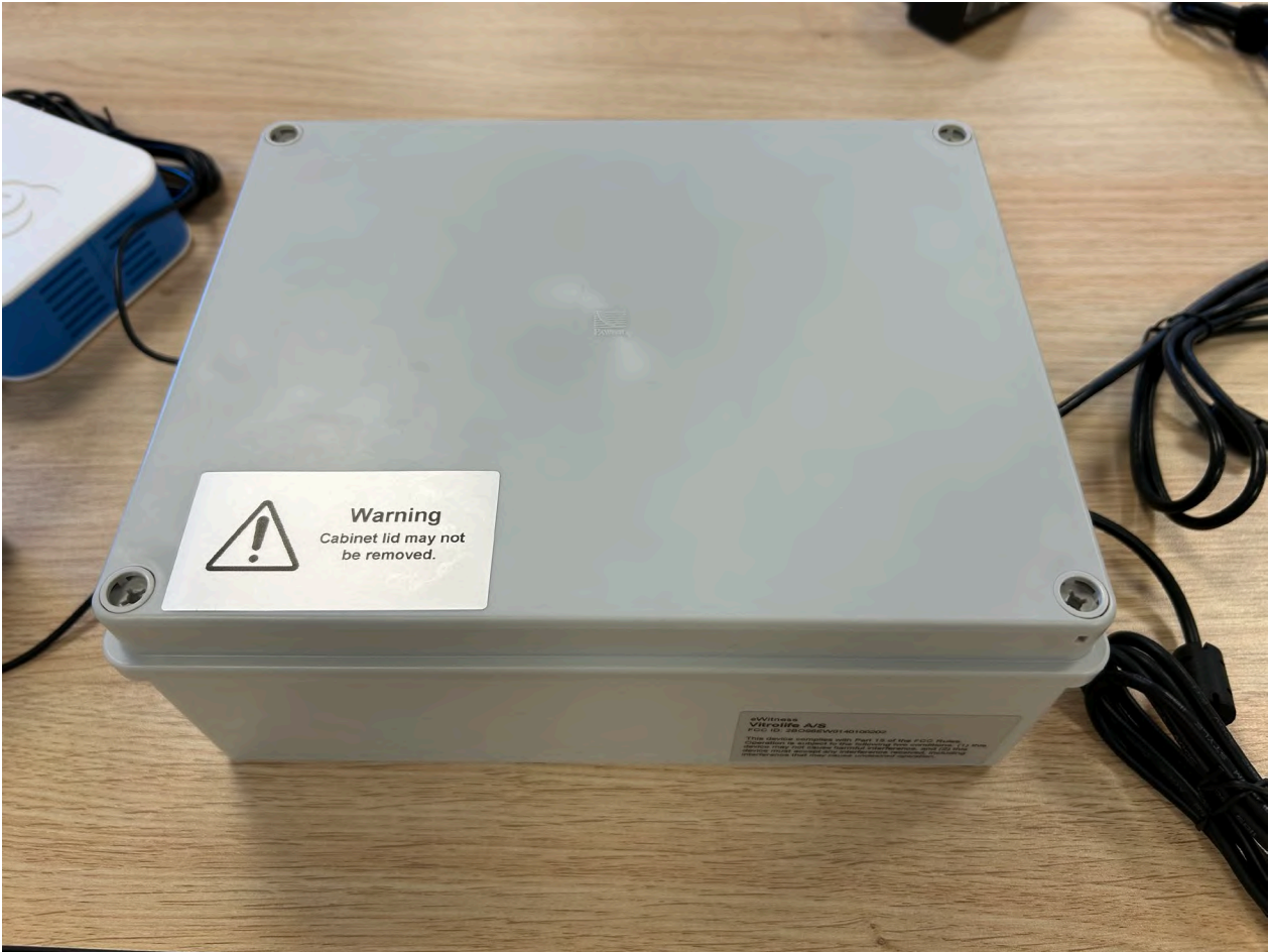
RFID reader in cabinet close up view from top with label placement
