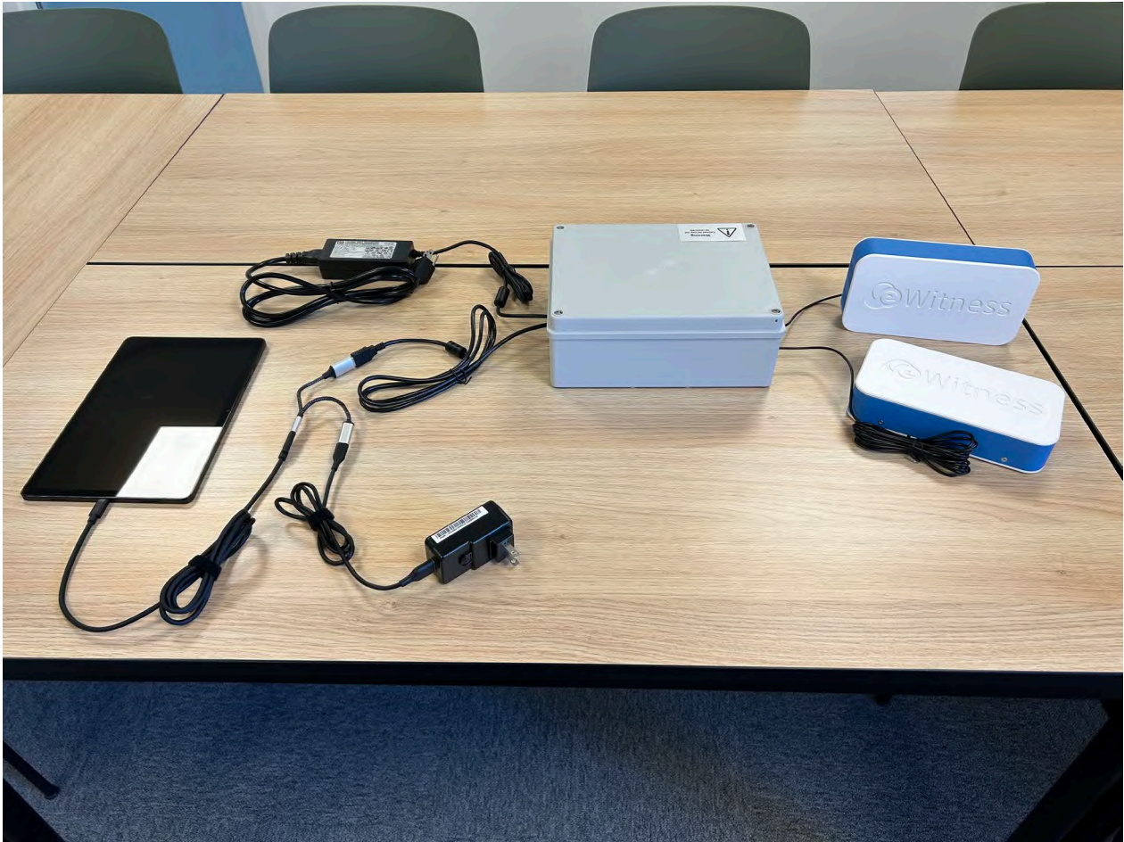
System picture from front view with lid on RFID reader in cabinet.
