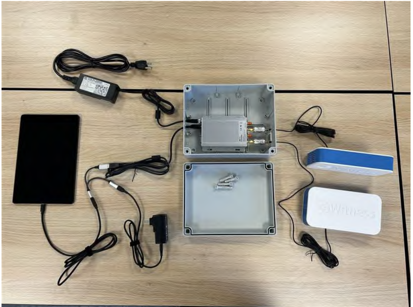
System picture from top, with no lid not mounted on the RFID reader in cabinet.
