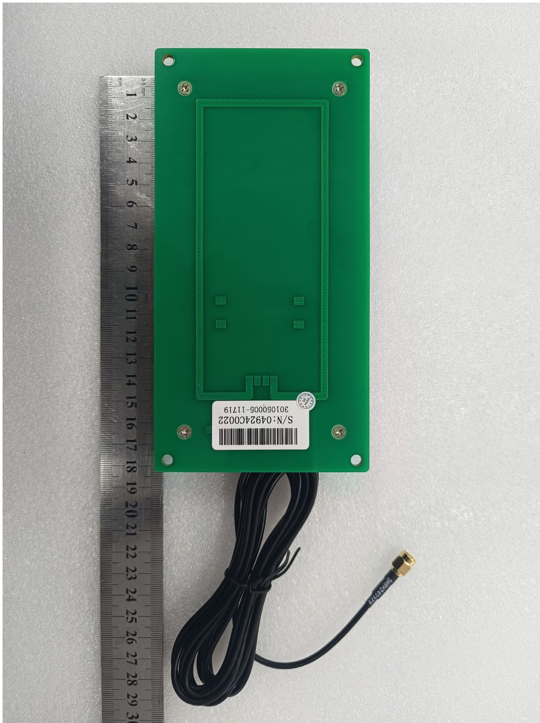
HF RFID Shielded Antenna EA2602-BL-P PCB Picture from bottom view 1 rev 10.03
