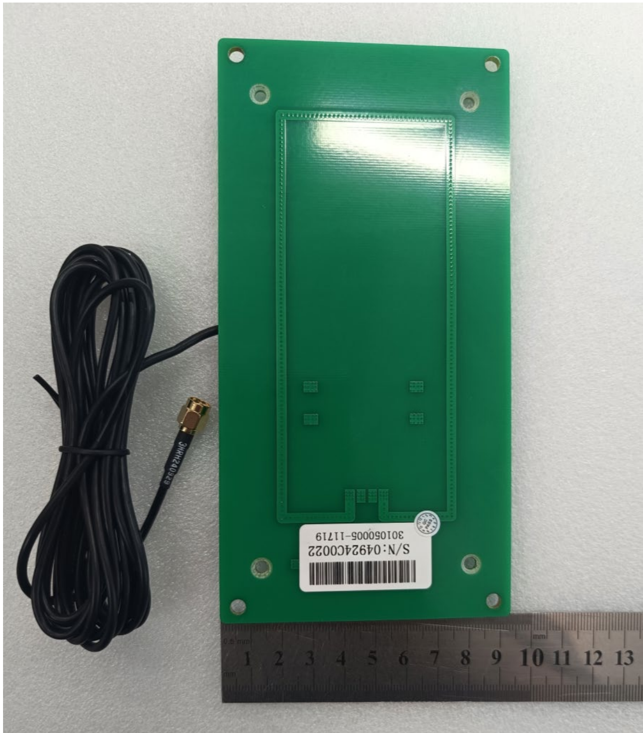
HF RFID Shielded Antenna EA2602-BL-P PCB Picture from bottom view 3 rev 10.03
