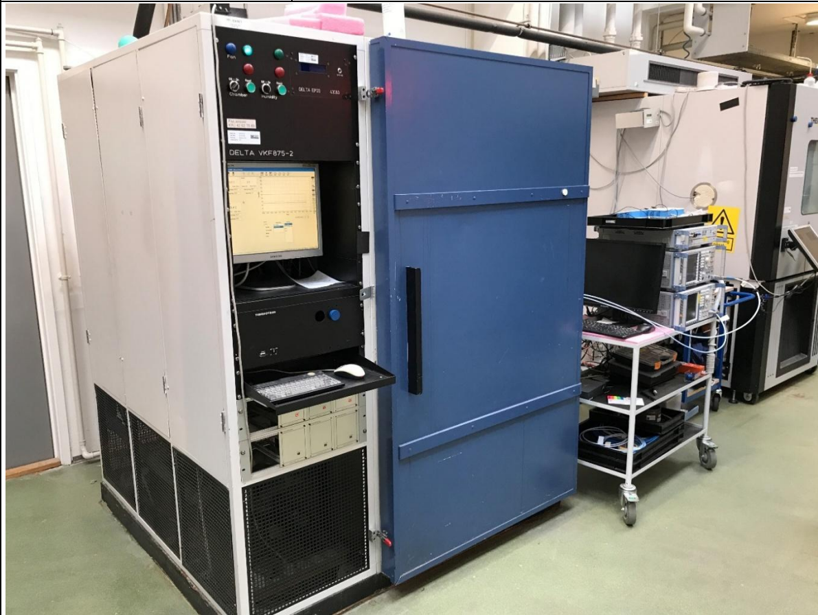
Photo 4.5.3 .....: Measurement of frequency stability with respect to ambient
