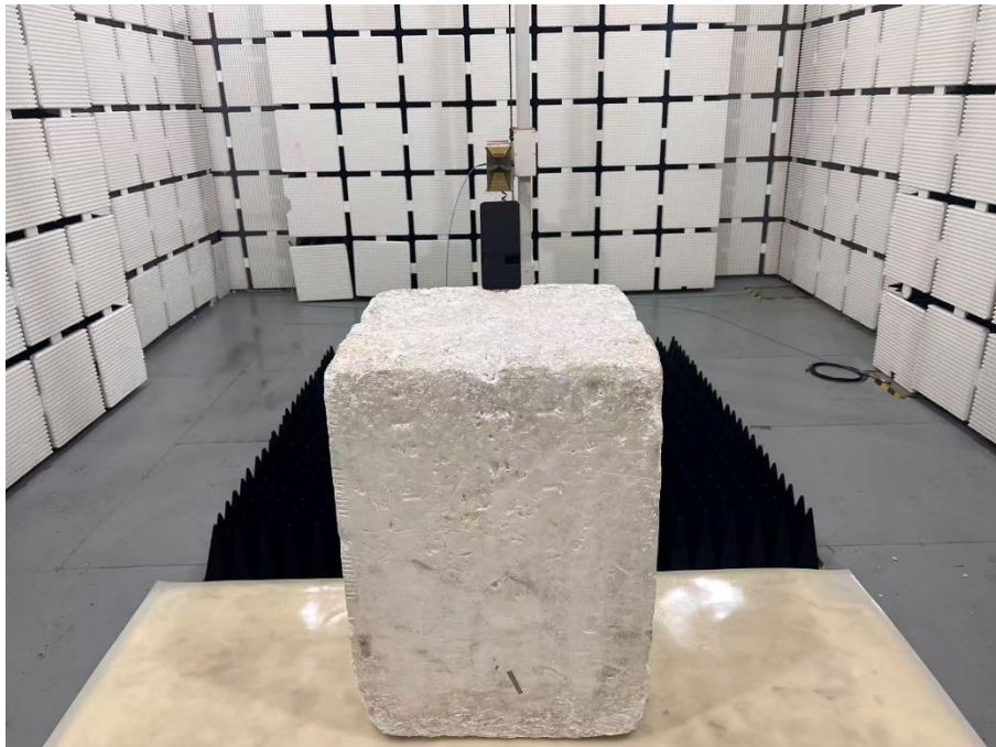
Set-up for Radiated Spurious Emission, Above 1GHz
