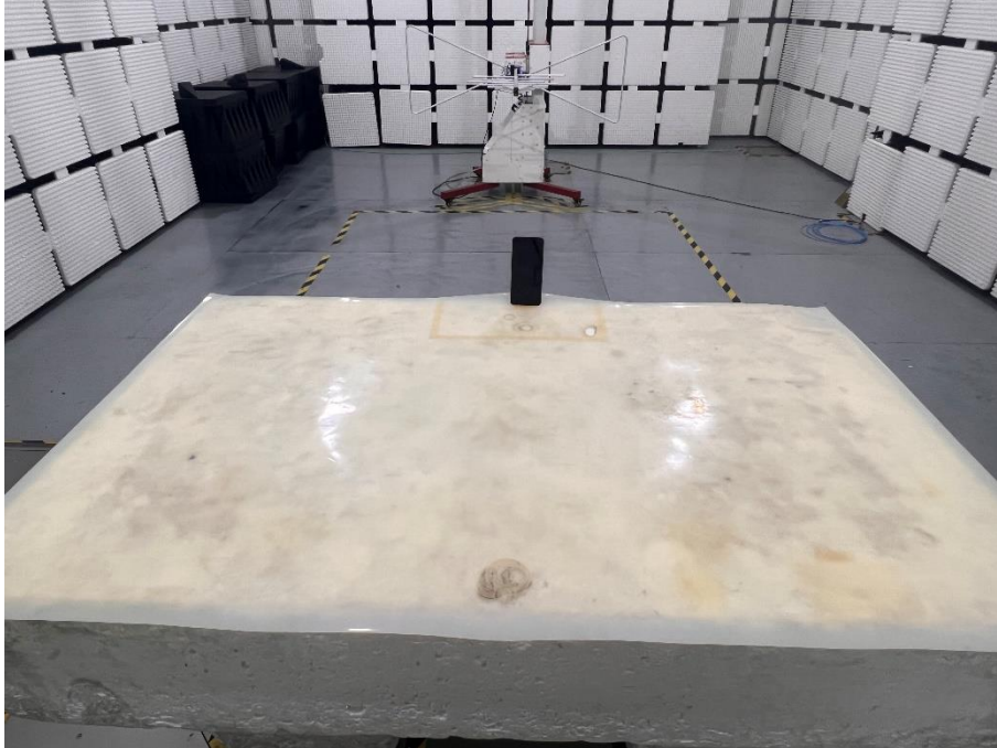
Set-up for Radiated Spurious Emission, Above 1GHz
