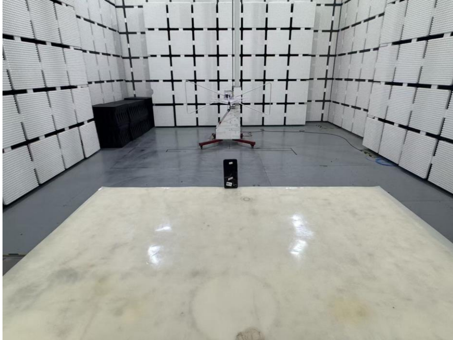
Set-up for Radiated Spurious Emission, Above 1GHz
