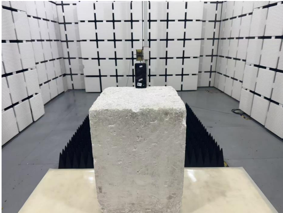
Set-up for Radiated Spurious Emission, Above 1GHz
