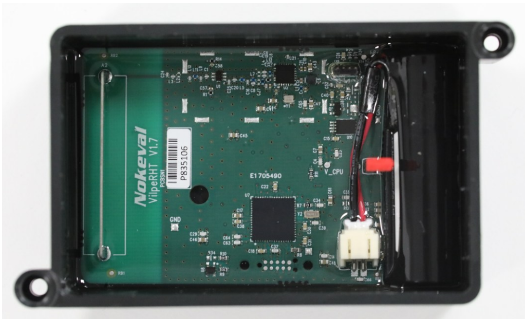
complete device, back cover open, potted
