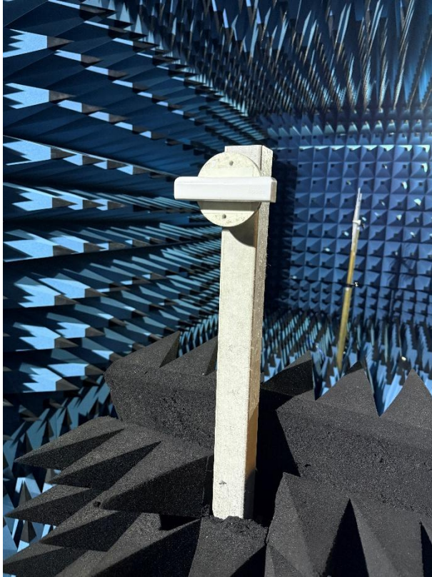
figure 2: DUT mounted on antenna rotating stand, battery powered
