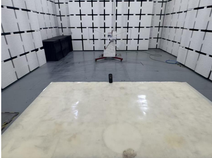
Set-up for Radiated Spurious Emission, Above 1GHz
