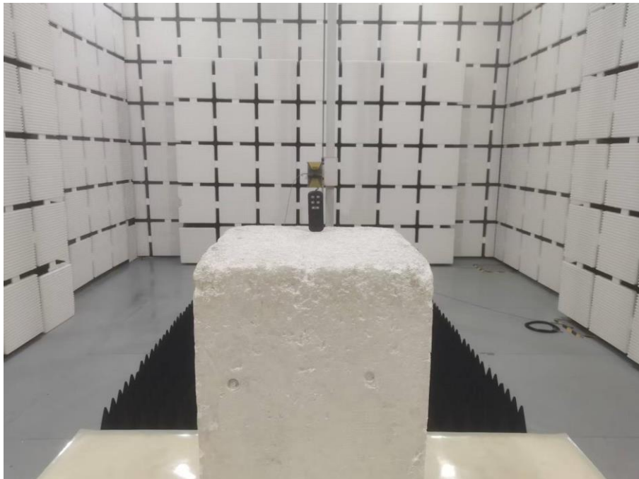
Set-up for Radiated Spurious Emission, Above 1GHz
