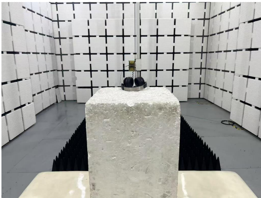
Set-up for Radiated Spurious Emission, Above 1GHz
