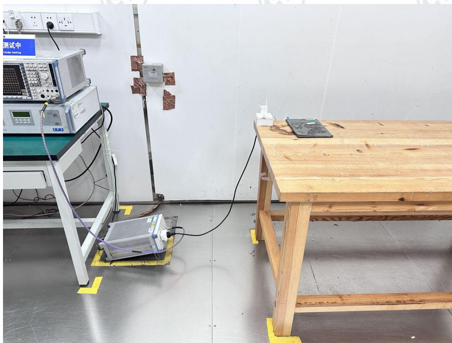
Conducted Emissions Test Setup
