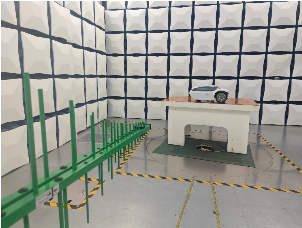
Test Set-up: Radiated spurious emission 30MHz-1GHz
