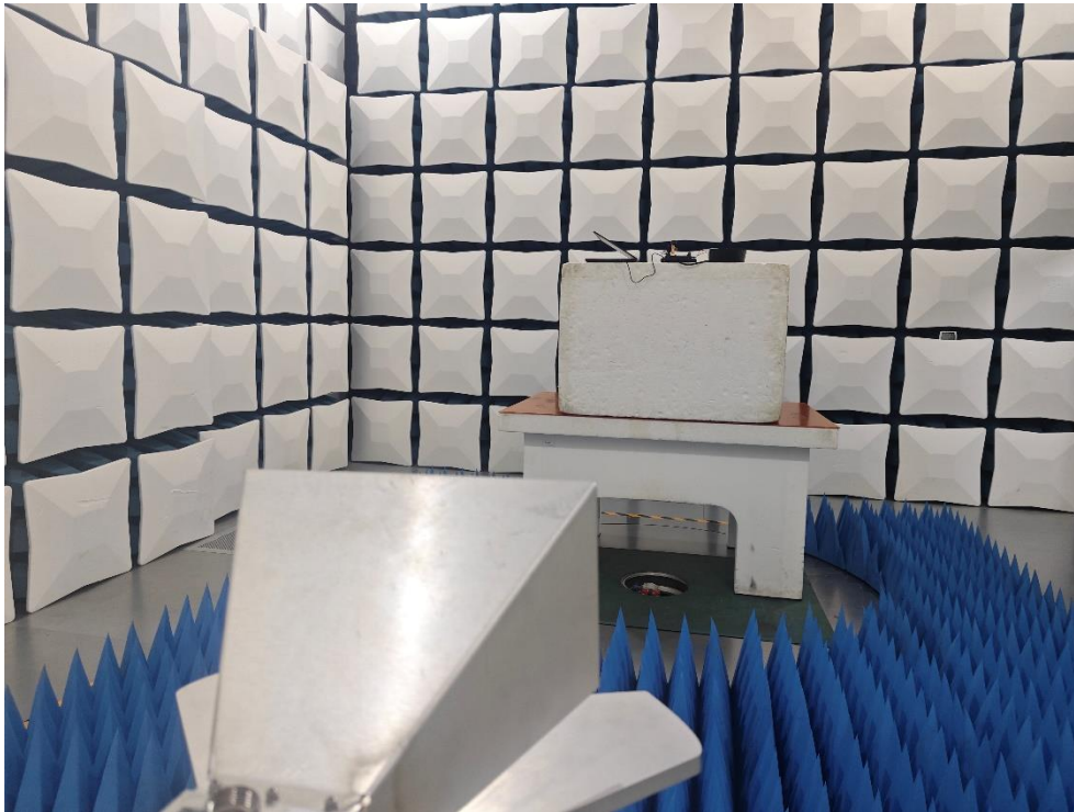
Test Set-up: Radiated spurious emission Above 1GHz
