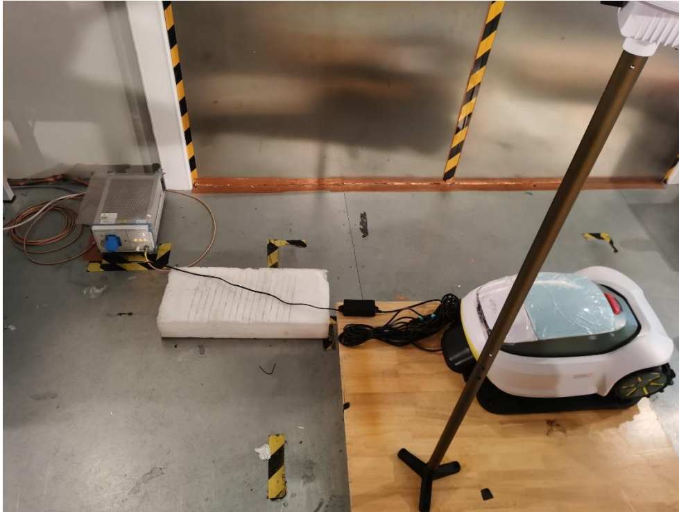
Test Set-up: Conducted emission 150KHz-30MHz
