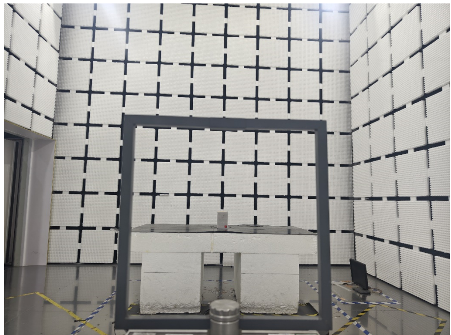
Radiation Emission Test Setup (Below 30MHz)
