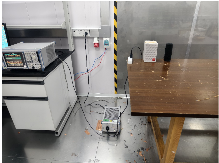
Conducted Emission Test Setup
