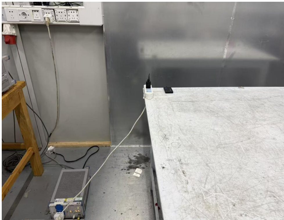
Description: AC Conducted Emissions Test Setup
