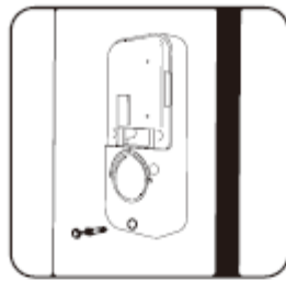
Fix interior assembly with interior screws
