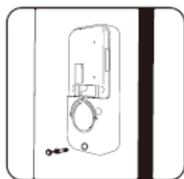
Fix interior assembly with interior screws
