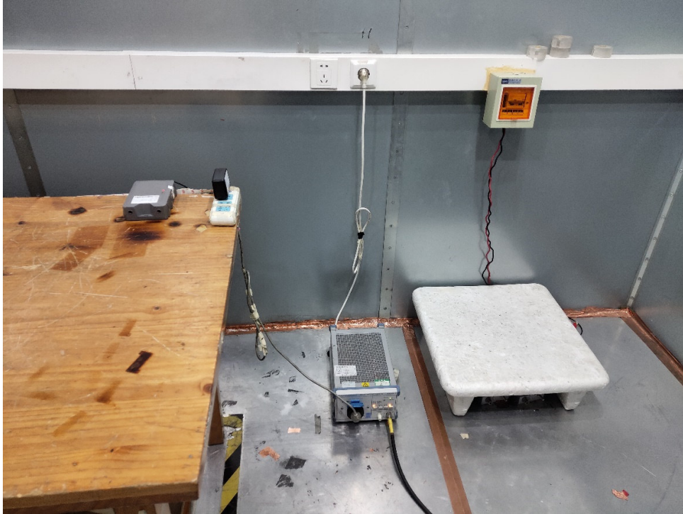
Picture 2: Conducted Emissions Test Setup
