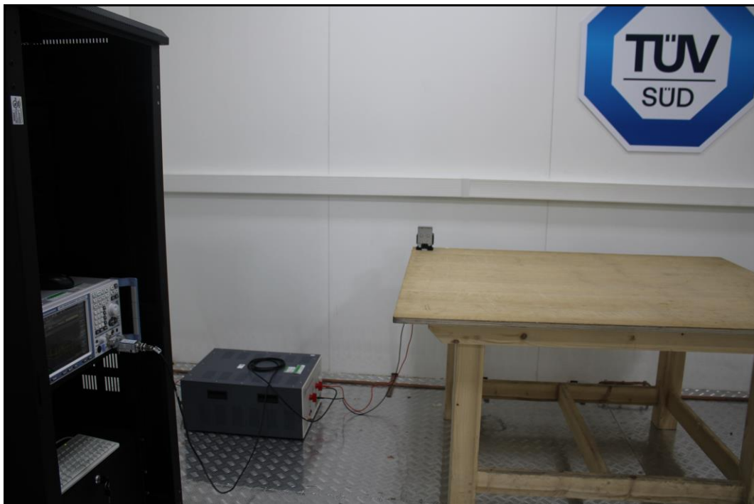
Conducted AC Power Lines Test Setup
