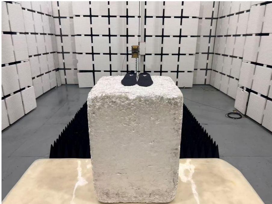
Set-up for Radiated Spurious Emission, Above 1GHz
