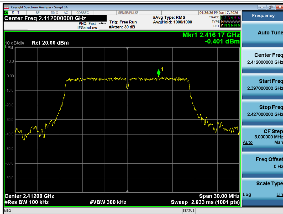
Tx. Spurious NVNT g 2412MHz Ant1 Ref
