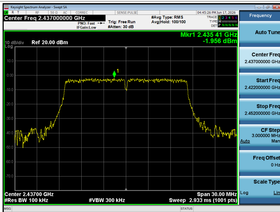
Tx. Spurious NVNT g 2437MHz Ant1 Ref
