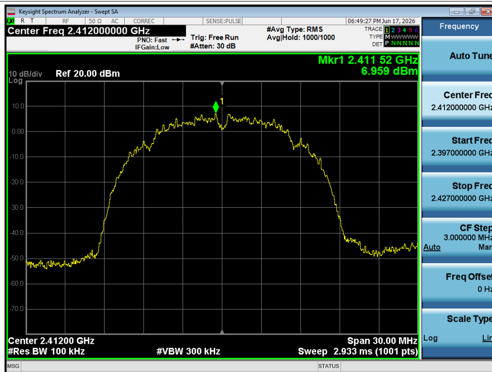
Tx. Spurious NVNT b 2412MHz Ant1 Ref
