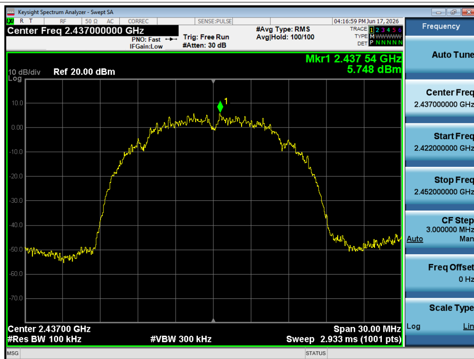
Tx. Spurious NVNT b 2437MHz Ant1 Ref
