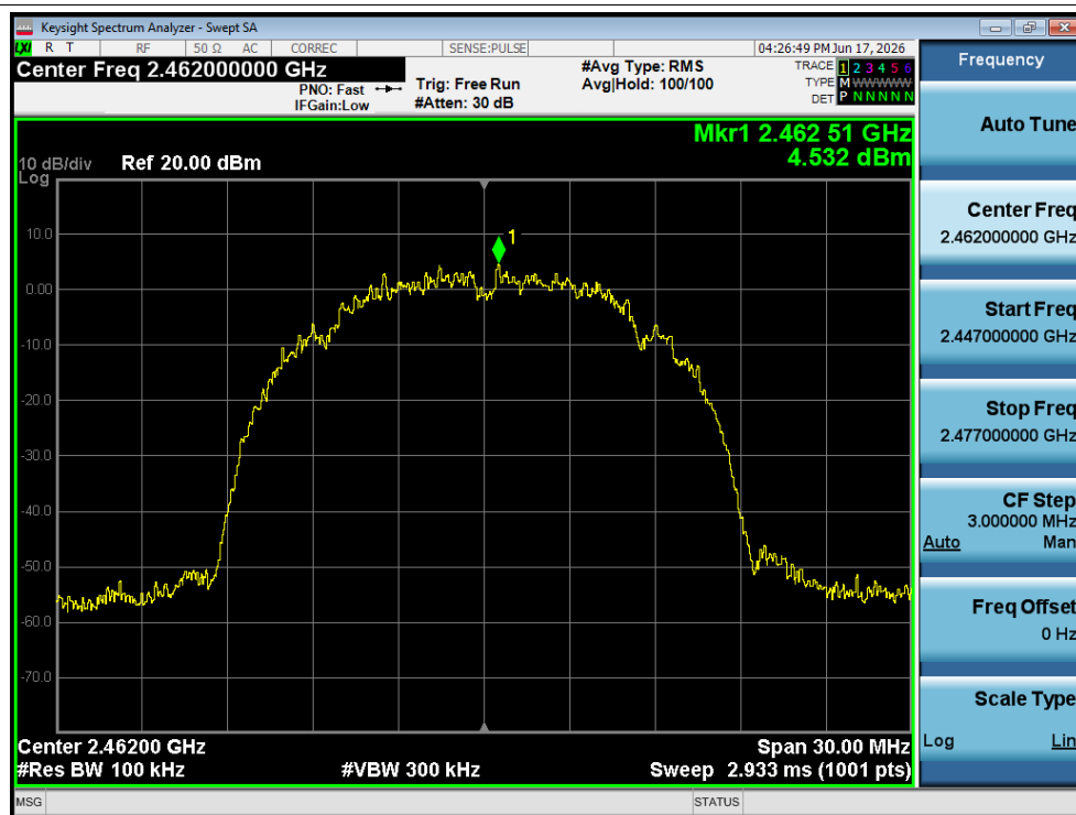
Tx. Spurious NVNT b 2462MHz Ant1 Ref
