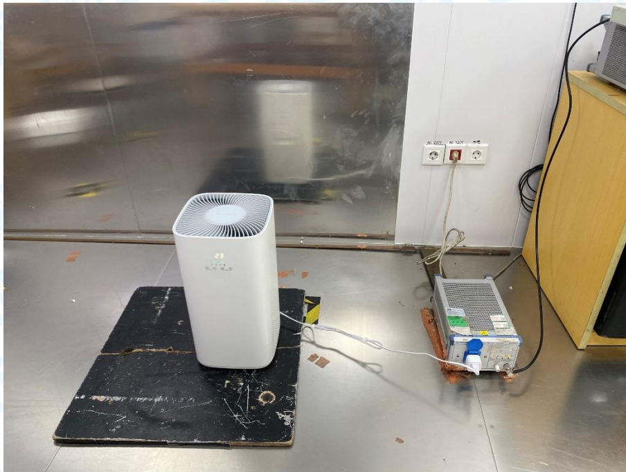
Photo of Setup for Conducted Emission
