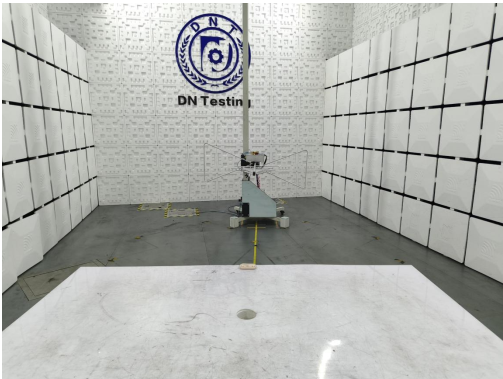
Radiated Emission Test View (Below 1G)
