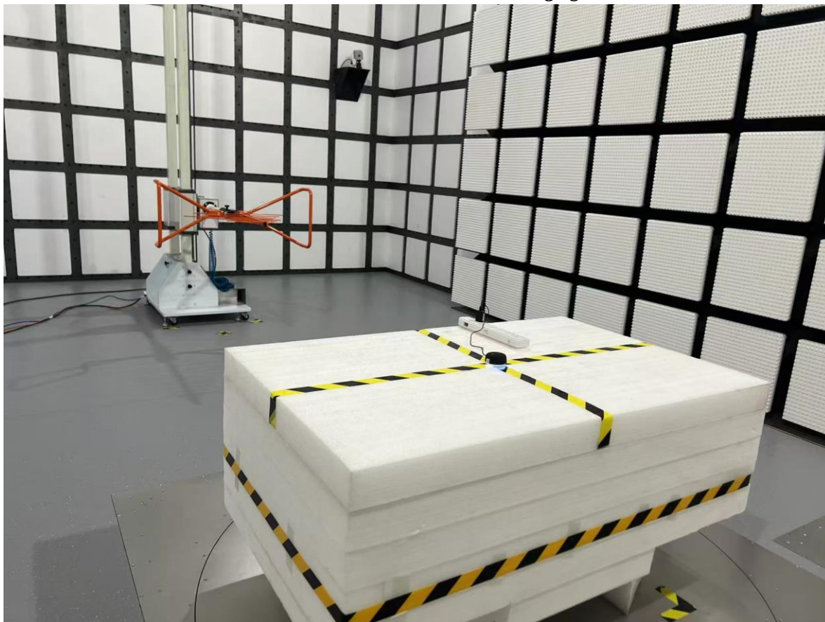
Radiated Emission 9 kHz-30 MHz Parallel View_Charging from USB
