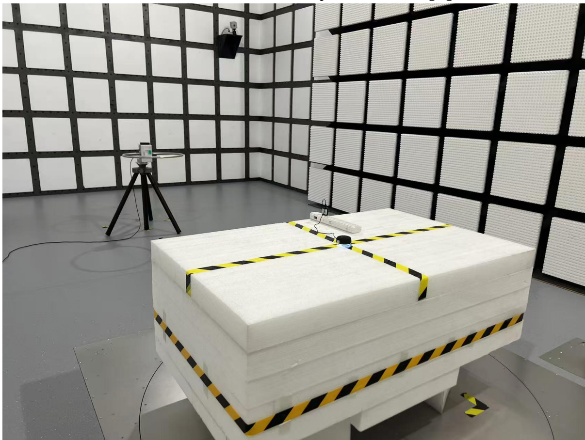
Radiated Emission 9 kHz-30 MHz Ground-parallel View_Charging from USB
