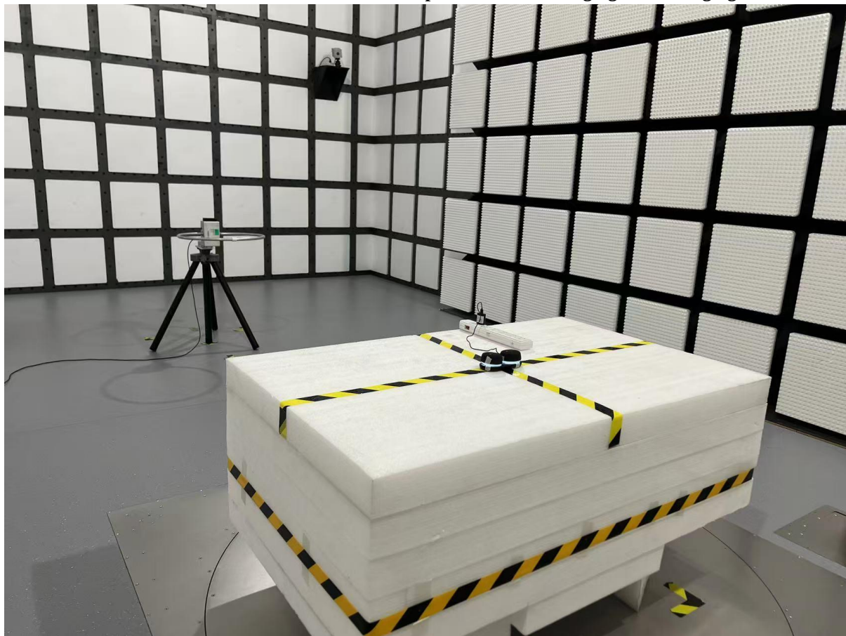
Radiated Emission 9 kHz-30 MHz Ground-parallel View_Charging from charging base
