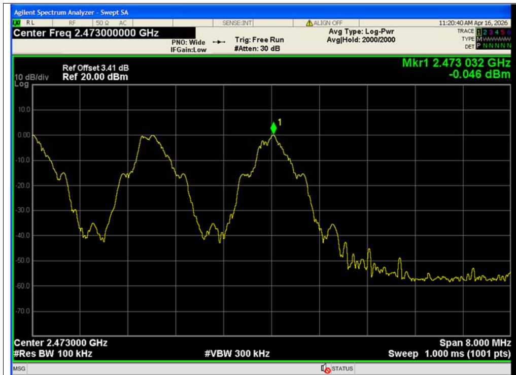
Band Edge(Hopping) NVNT 2.4G 2473MHz Ant1 Hopping Ref
