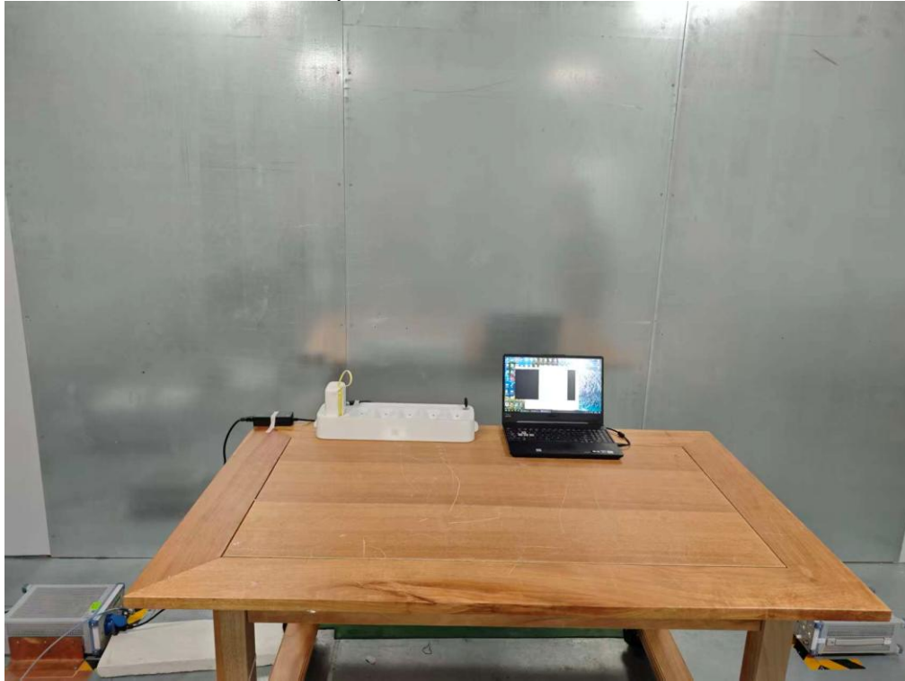
Conducted Emission Setup at AC Power Line
