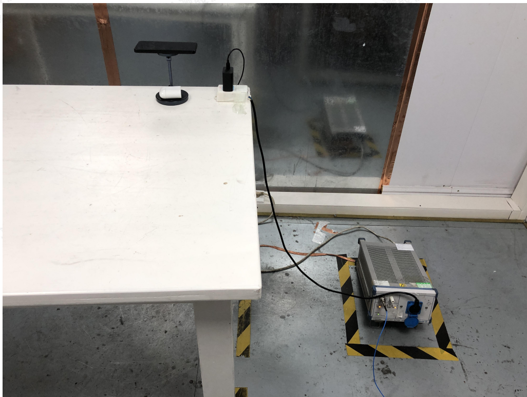
Conducted Emission-AC adapter charge mode
