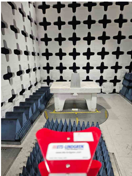
Radiated emissions test set up above 18GHz.
