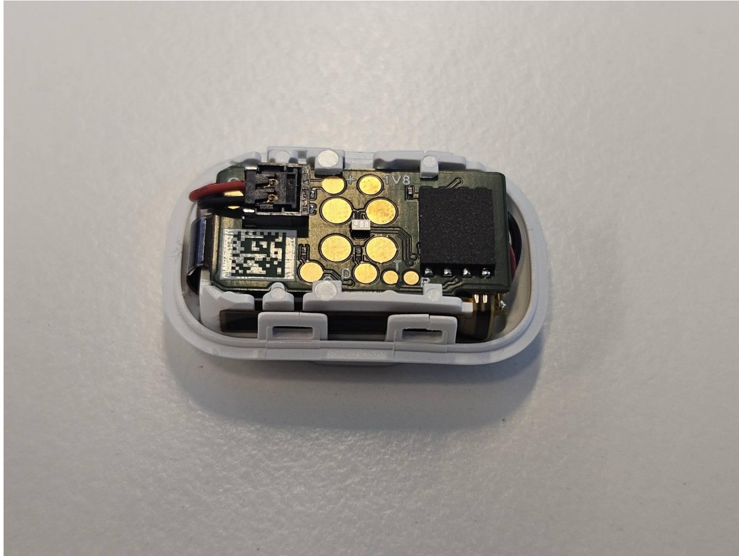
Frame assembly inside bottom cover
