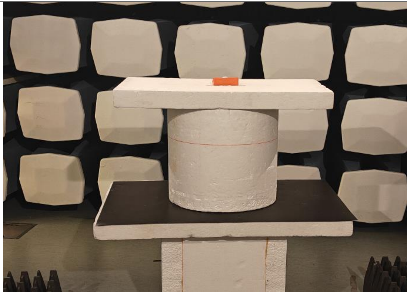
Picture 12, Radiated Spurious Emissions, EUT setup, TX 1 – 26 GHz
