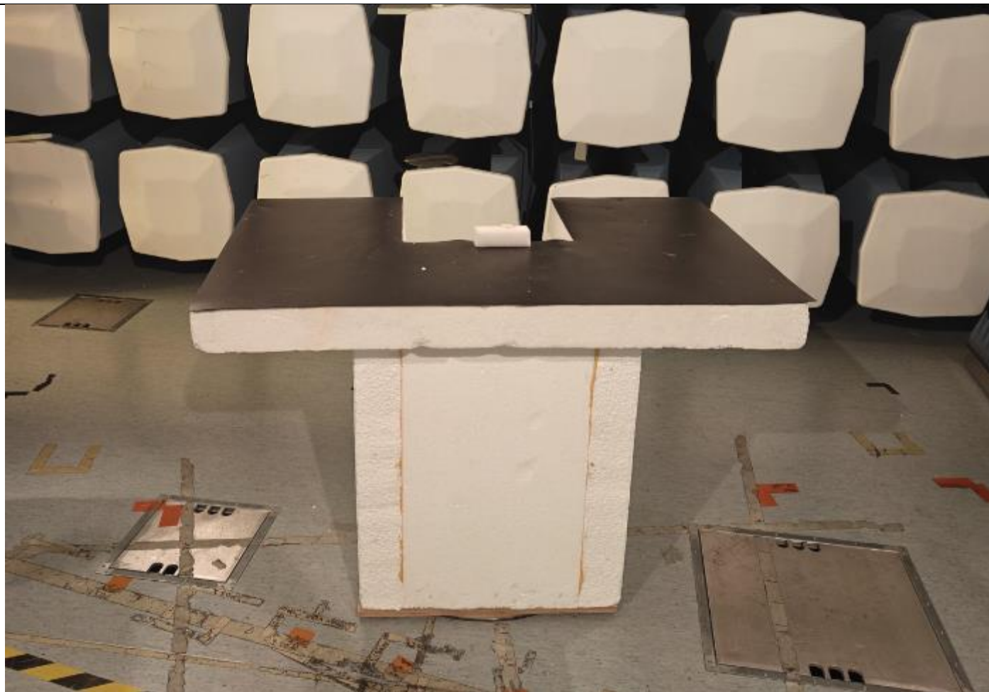
Picture 11, Radiated Spurious Emissions, EUT setup, TX and RX 30 – 1000 MHz
