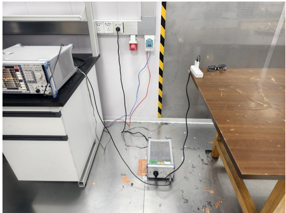
Conducted Emission Test Setup
