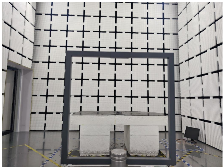
Radiation Emission Test Setup (Below 30MHz)
