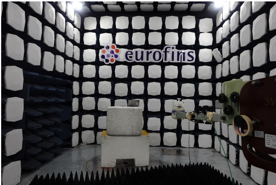
Picture 1 Radiated Emission Test Setup
