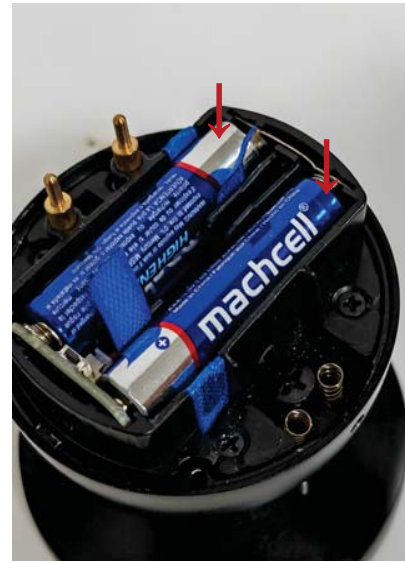
11. Install two more batteries
