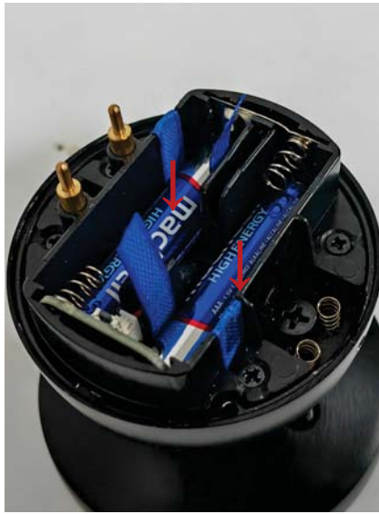
10. Install the next two batteries
