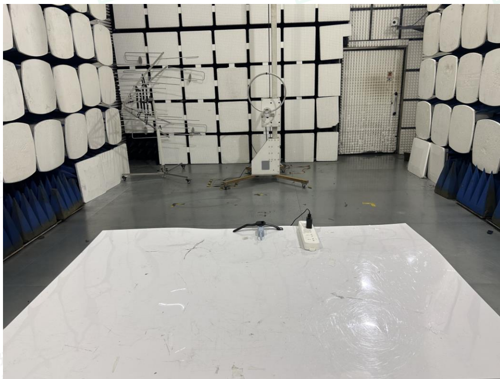
Radiated Emission below 30MHz-AC adapter charge mode
