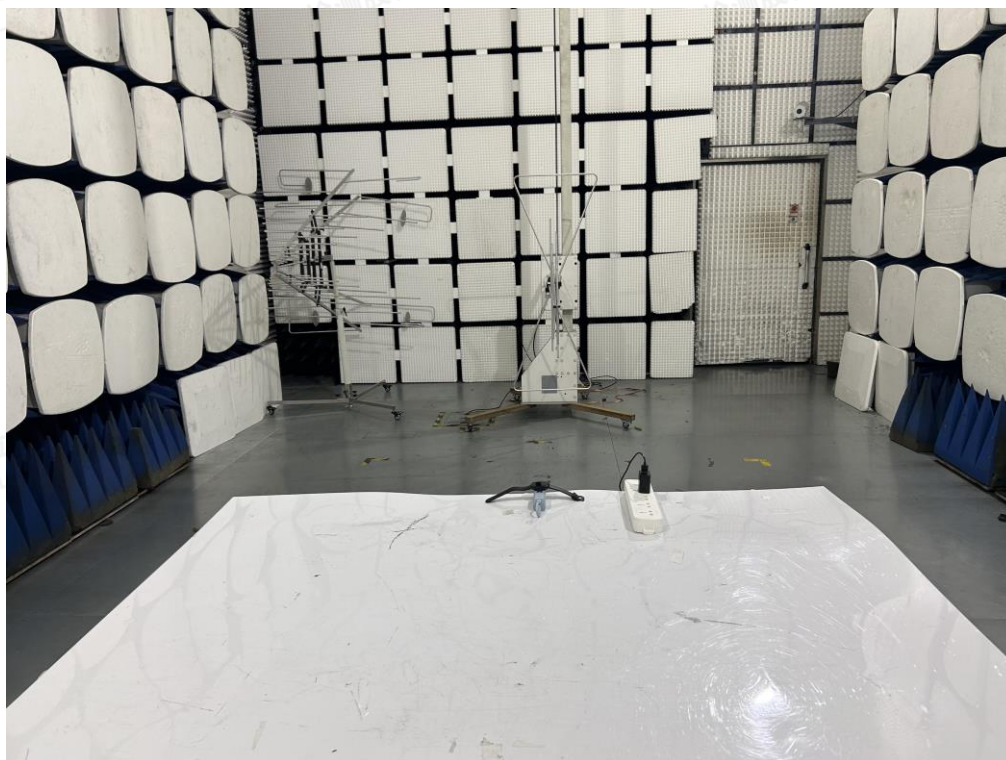
Radiated Emission below 1GHz-AC adapter charge mode
