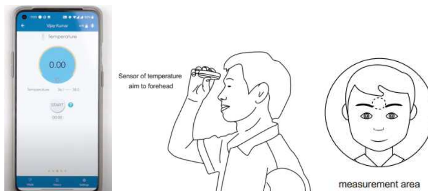
Fig. 9 Temperature vital screen, positioning of sensor for measurement and measurement area
