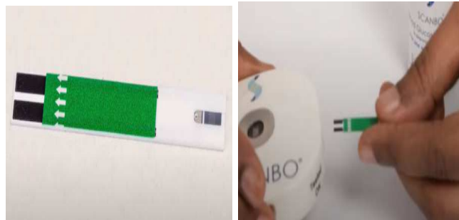
Fig. 15 Glucose Test Strip and its insertion into the device
