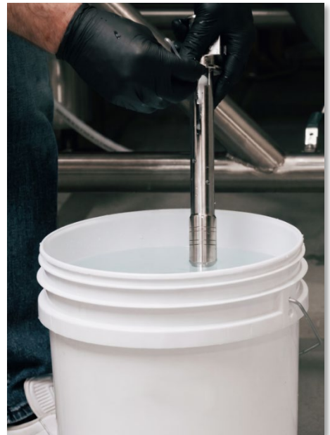
Figure 6 -1: Cleaning the M3 - Proper Submerging Depth
